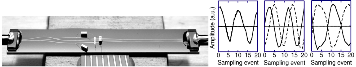
Fig. 1. 90° waveguide optical hybrid (left). The sources are input on the left, split and recombined into 4 outputs on the right. The relative phase between the two quadratures can be set using a thermo-optic phase shifter, and examples of quadratures measured for phase differences equal to 0, \pm \pi/2 and \pi are plotted on the right.
